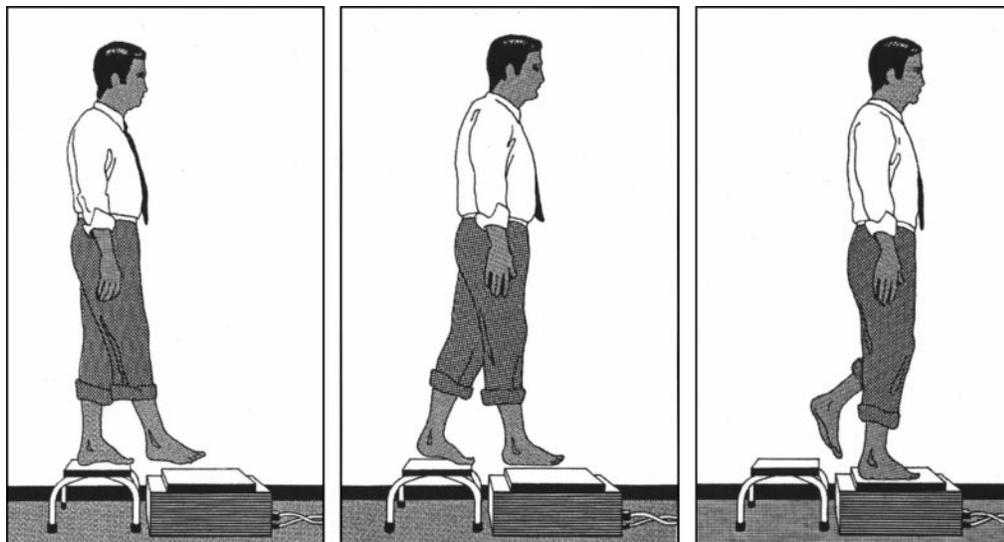
Fig 1. Schematic representation of testing set-up for impact measurement. Subjects stepped down onto the force platform and balanced on 1 foot after contact with the platform. Subjects were tested barefoot, with gaze straight and arms at side on landing.
